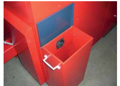
↑ Automatic ash removal container
