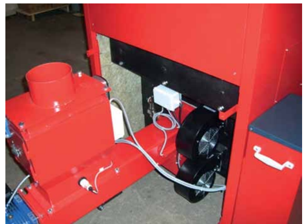
↑ Spring mounted air valve prevents burn back, infrared level detector and fans for the combustion air.
