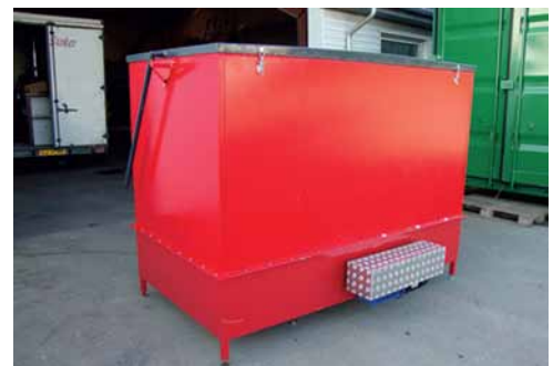
Prefabricated hopper manufactured from steel panels.
