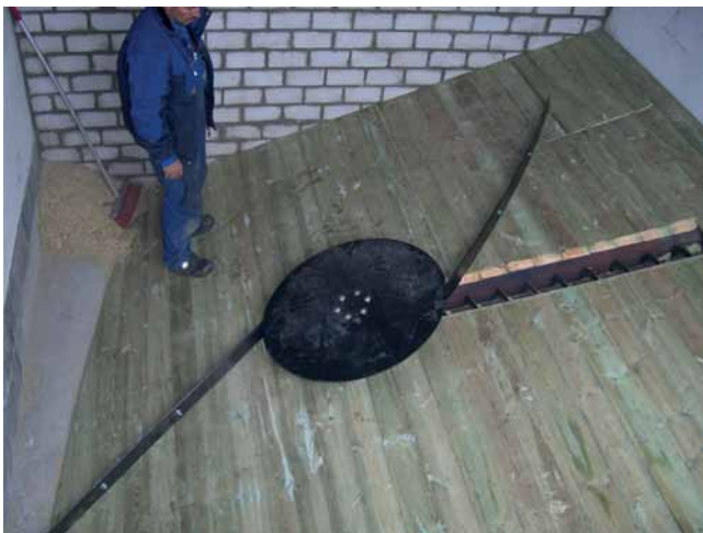
Sweep auger. Walls and floor are constructed onsite (not included in equipment supplied by KSM)
