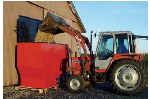
Prefabricated hopper manufactured from steel panels.
